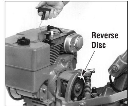
Figure 5-25: Checking Reverse Disc in NEUTRAL.
